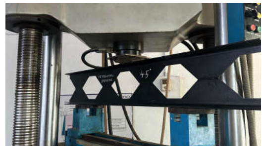
Fig. No:-3 Testing of Castellated beam with 45° Opening
