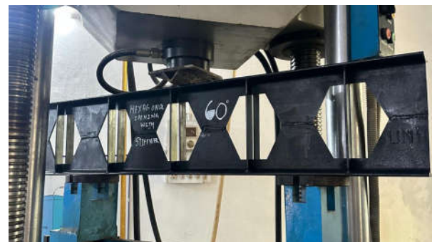
Fig. No:-19 Testing of Castellated beam with stiffeners & 60° Opening
