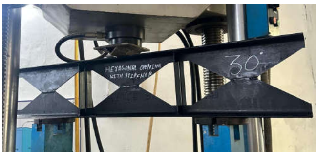
Fig. No:-4 Testing of Castellated beam with stiffeners & 30° Opening
